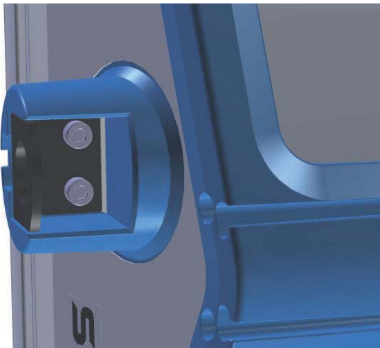
Figure 7: To mount the safety loop brackets
