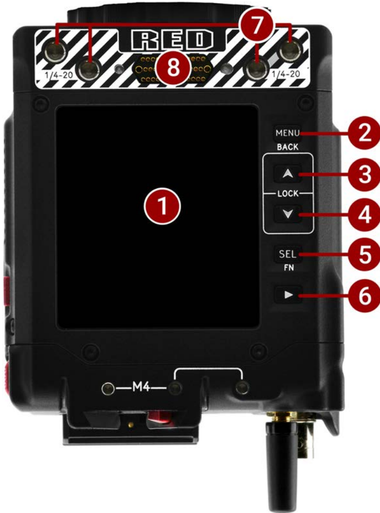
Figure: Camera Body Top Controls and Features
