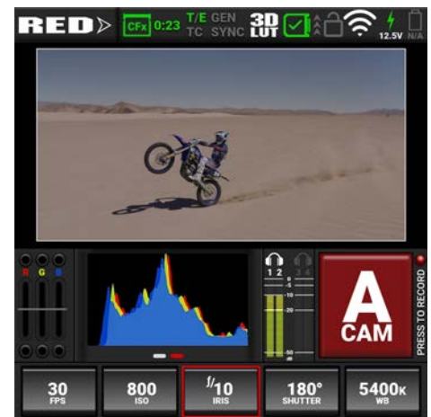
Example of a balanced exposure with histogram and exposure meter:
