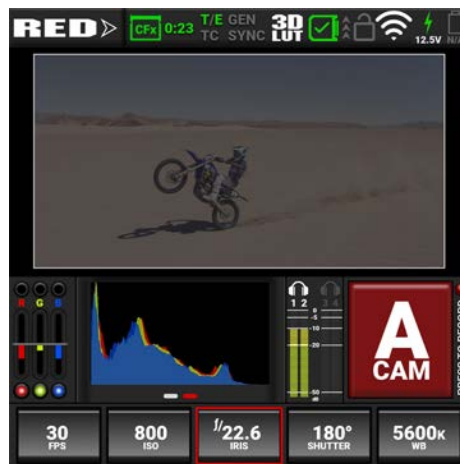
Example of underexposure with histogram and exposure meter:
