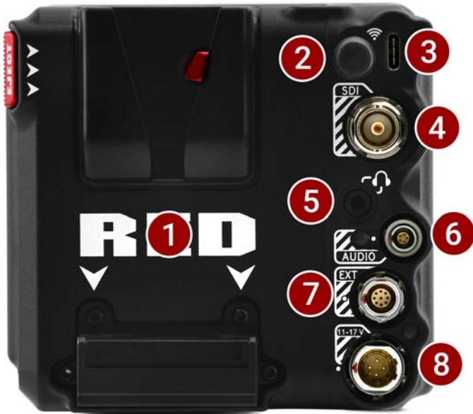
Figure: Camera Body Rear Controls and Features
