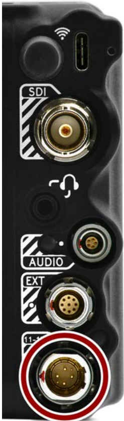
Figure: Front face of the male 6-Pin 1B DC power input connector (looking at the back of the camera).
